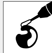
4. Shape the blank with special cutters (from page 169)
